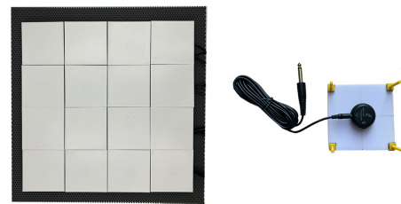
Figure 2: Fully assembled miniature mounted in foam, which serves as a surface for capturing sound (left), and an individual module displaying the contact microphone embedded in the center (right).
